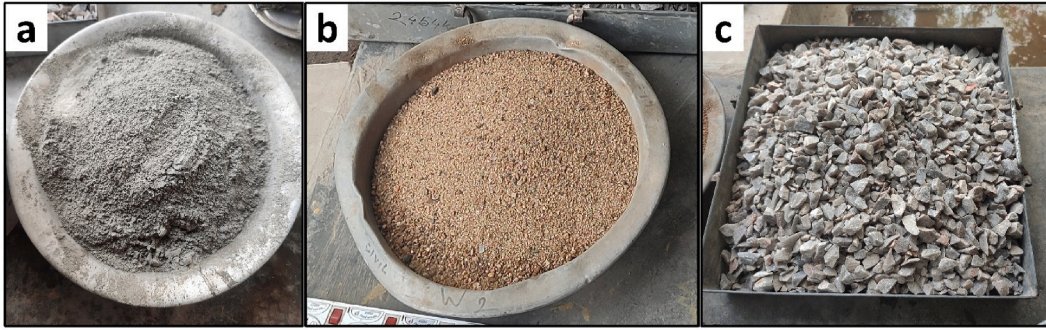
Fig. 2. Samples of raw materials used: (a) OPC, (b) fine aggregate, and (c) coarse aggregate.
