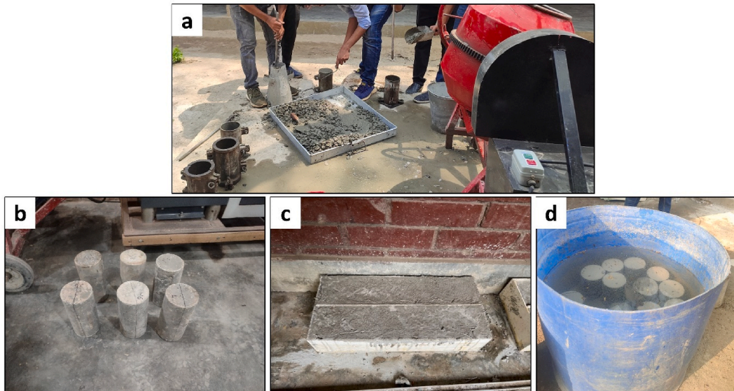
Fig. 5. Preparation of concrete specimens: (a) casting, (b) cylindrical, and (c) prism specimens, and (d) curing method.
