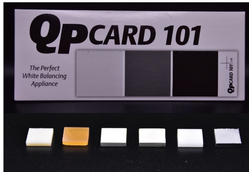
Figure 1. Substrate material. The upper row is the QP Card (white, gray, and black); the lower row shows CR, MR, PEEK, PEKK, Y-TZP, and Co-Cr in that order.
