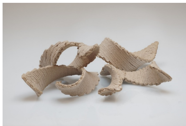
Figure 6. 3D printed wood warped seedpod. These were made by printing to helical ribbons of opposite chirality with a relative angle of 45°.
