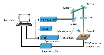
Figure 1. The device of laser-induced breakdown spectroscopy (LIBS).
