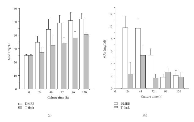
FIGURE 4. Comparison of MAb production rates between rolling DMRBs and T- asks. The MAb concentrations are measured in the medium supplemented with 5% FCS in both DMRBs and T- asks. (a) Accumulated MAb production. (b) Daily MAb production. The values are mean SD of three independent experiments. Vertical bars are SDs.
