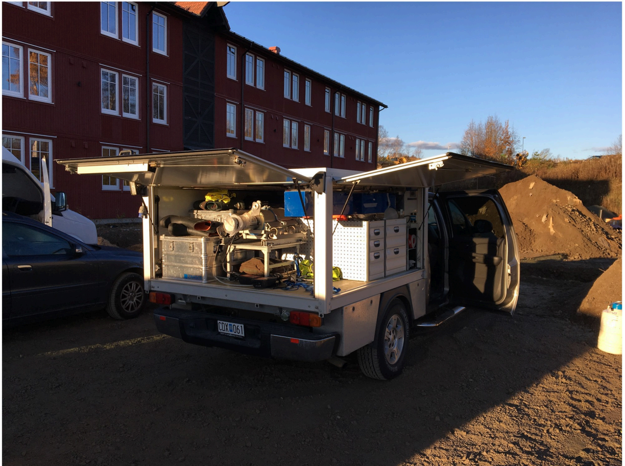
Fig 4. A picture of the open flat bed portion of the mobile gamma spectrometry vehicle used in the experiment. The 123% HPGe detector with its dewar can be seen in the back of the flat bed, with the active medium of the detector pointing to the back of the vehicle. The two blue boxes in the top of the right side of the flat bed are the 4l NaI(Tl) detectors. The rear pillars of the flat bed structure can be also clearly seen.
