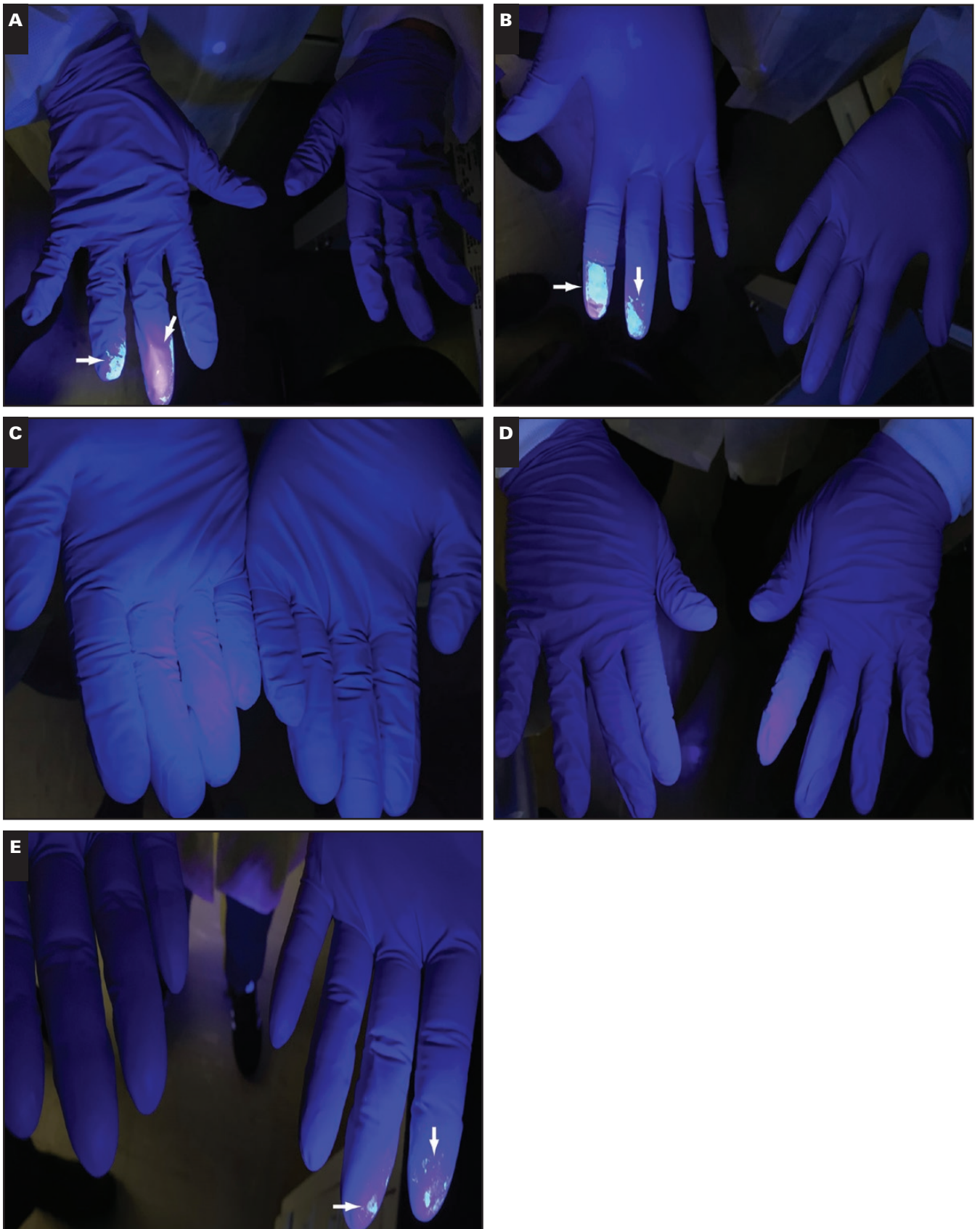
Figure 1 ID NOW visualization of Glo Germ cross-contamination following mock sample handling. Representative of users' gloves after processing mock Glo Germ sample on the ID NOW. Contamination zones denoted by arrows. A , User 1, laboratory staff. B , User 2, nonlaboratory staff. C , User 3, laboratory staff. D , User 4, nonlaboratory staff. E , User 5, laboratory staff.
