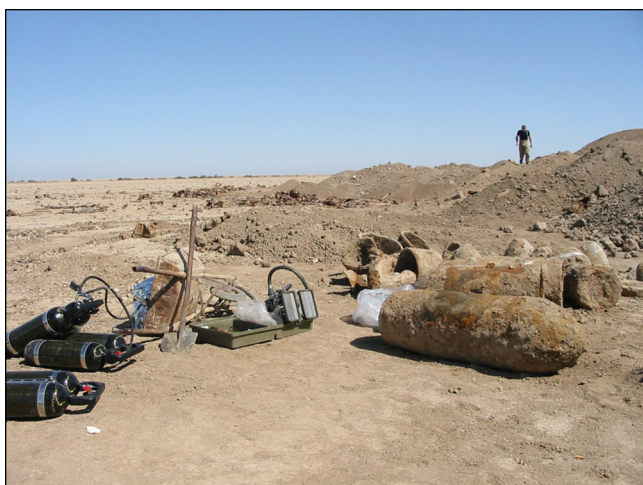
FIG 4 Excavated R400 bombs from Al Azizia site. On the left of the photo is the drilling prototype device called MONICA. (Photo taken by Kay Mereish.)
