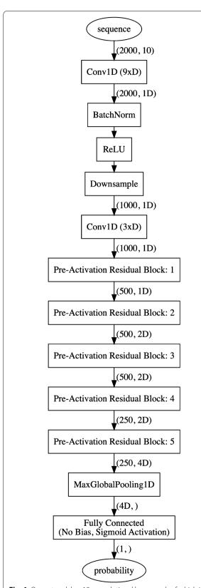
**Fig. 4** Our network has 12 convolutional layers, each of which is followed by batch normalization and a rectified linear unit. Residual connections are used to improve gradient propagation throughout the network
