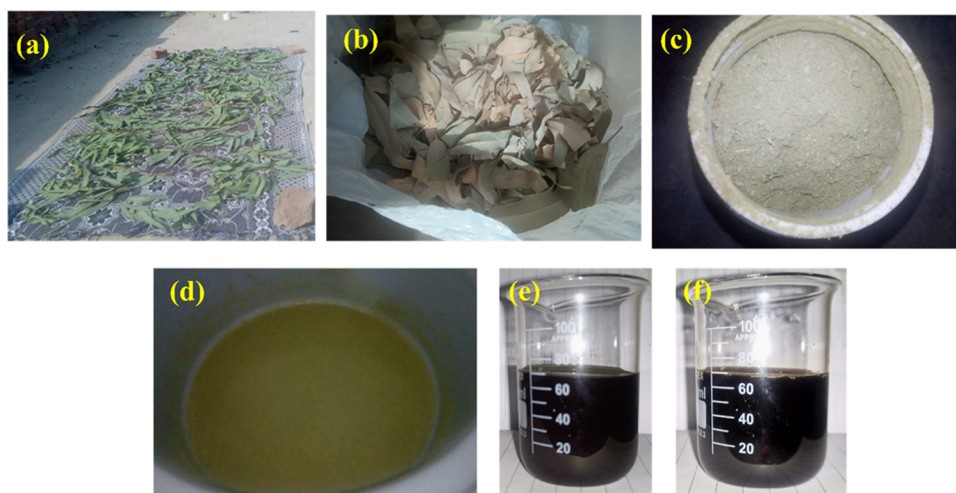
Figure 2. Steps involved in extraction of eucalyptus-based natural finish: (a) eucalyptus green leaves, (b) dried leaves, (c) powdered eucalyptus leaves, (d) powdered eucalyptus leaves in water, (e) eucalyptus and water extract unheated, and (f) eucalyptus and water extract heated.
