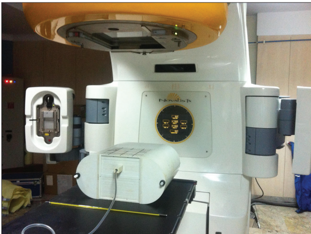
Figure 1: Cylindrical phantom used for point dose measurements with Rapid Arc for 10 patients
