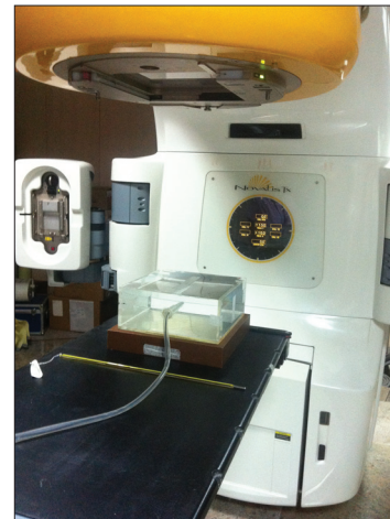
Figure 2: Rectangular phantom used for point dose measurements with Rapid Arc for 10 patients
