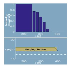
**Figure 9.** Merging section of I-101 and inequality constraints. The upper plot presents the inequality constraints setting as a function of the distance till the end of the merging section, whereas the lower figure gives a graphical description of the merging section.
