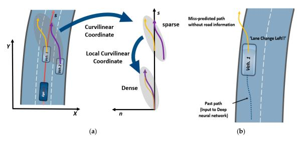
**Figure 2.** Practical problem statement. (a) If we represent trajectories of the surrounding vehicles in the local curvilinear coordinate system, the data distribution becomes compact; (b) Wrong prediction is caused by a zigzag motion of the vehicle without any road constraint.
