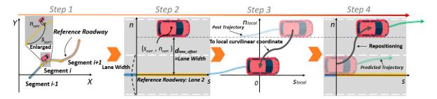
**Figure 5.** Description of the data processing steps. Step 1: Global Cartesian coordinates; Step 2: Transformation to the curvilinear coordinates; Step 3: Translation to the local curvilinear coordinates; Step 4: Repositioning to the curvilinear coordinates.
