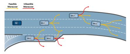
**Figure 1.** Schematic showing the concept of road-aware trajectory prediction: vehicles should run along roadway while obeying the structural constraints of the road.
