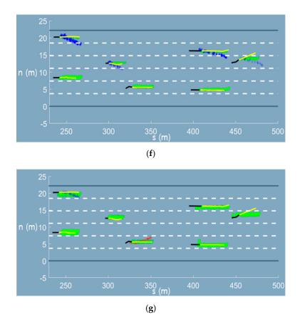
**Figure A2.** Comparative results of the trajectory prediction network. (**a–g**) are the results obtained by learning from 5%, 10%, 15%, 20%, 40%, 60%, and 80%, respectively, of the training dataset. The bigger and more apparent the marker, the higher the confidence level of the maneuver.
