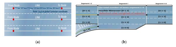
**Figure 3.** Extraction of road information. (a) HD maps contain nodes and links and each component is represented by points in the Cartesian coordinate system; (b) After extracting information via offline preprocessing, each segment has information corresponding to the segments such as B-spline parameters, lane information, length of the segment, and a feasible maneuver one-hot vector.
