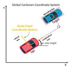
**Figure 4.** Global Cartesian coordinate system and body-fixed coordinate system for the representation of vehicle states.
