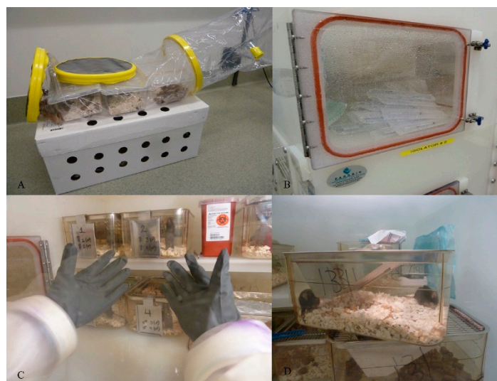
Figure 2. Sterility flow. (a) Shipment box used to deliver mice in a sterile environment. Flexible boxes are sealed with layers of tape and contain up to three cages. (b) Sterile port, with a hermetic door. Specific protocols outline procedures for introduction of supplies. (c) Interior gloves worn on top of sterile latex gloves to manipulate mice. (d) A cage with germ-free C57 BL/6 mice, containing specific autoclaved bedding, paper, food, and water.
