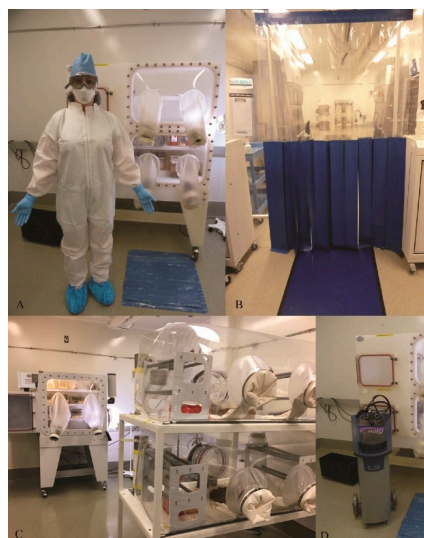
Figure 1. Equipment of the sterile environment (Bio-Bubble). (a) Personal Protective Equipment (PPE) required while using the Bio-Bubble: disposable coveralls, double shoe covers, double gloves, mask, double hair covers, goggles. (b) Antechamber dedicated to decontamination: sterile curtains separating antechamber and sterile room containing isolators and hood. (c) Sterile semirigid isolator, SRI, and flexible isolator. On the left of the SRI, port of entry, with sterile chamber for introduction of supplies. (d) Fogger (Quip) used to spray decontaminant inside the isolators and in the room prior to use.
