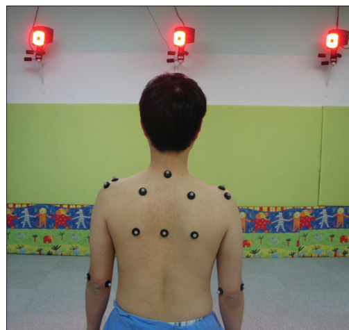
Figure 1: A clinical photograph showing a subject with attached reflective markers being examined using an optical tracking system, which is composed of six synchronized infrared cameras, allowing for 120-Hz data capture
