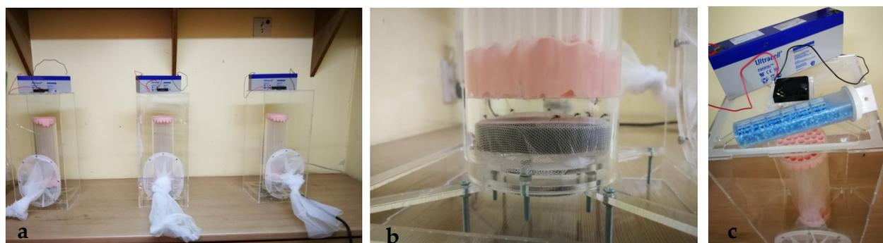
**Figure 1.** The flight capacity testing: (a) the simultaneous use of three IAEA flight devices. (b) The males introduced into the device cylinder. (c) The BG lure, energy source, and fan at the top of the device.
