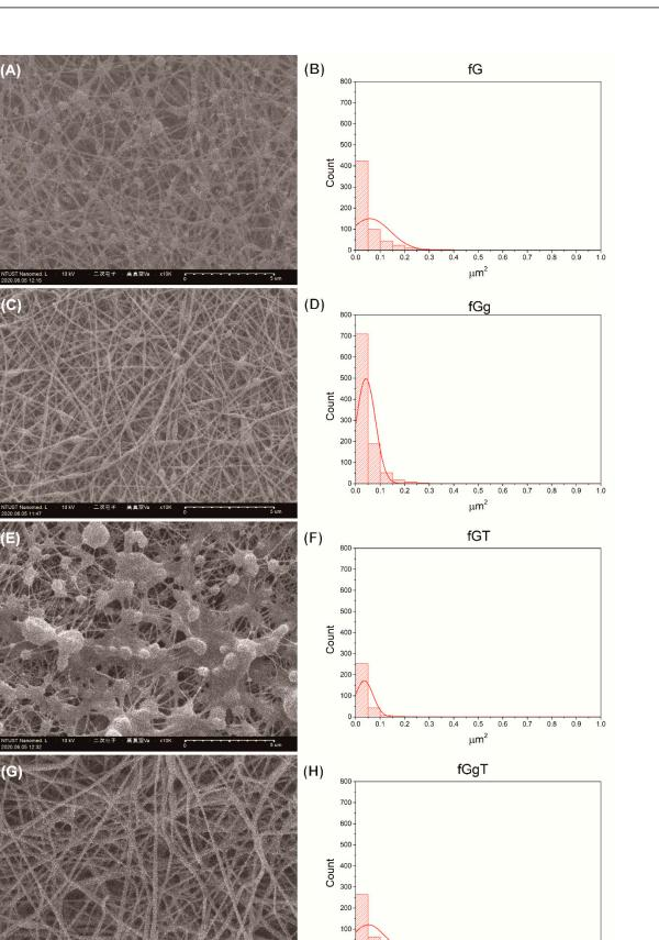
**Figure 2.** The SEM images of indicative nonwoven mat. (**A**,**B**) fG; (**C**,**D**) fGg; (**E**,**F**) fGT; (**G**,**H**) fGgT. (fG: fish gelatin, g: gallic acid, T: Tween 80).
