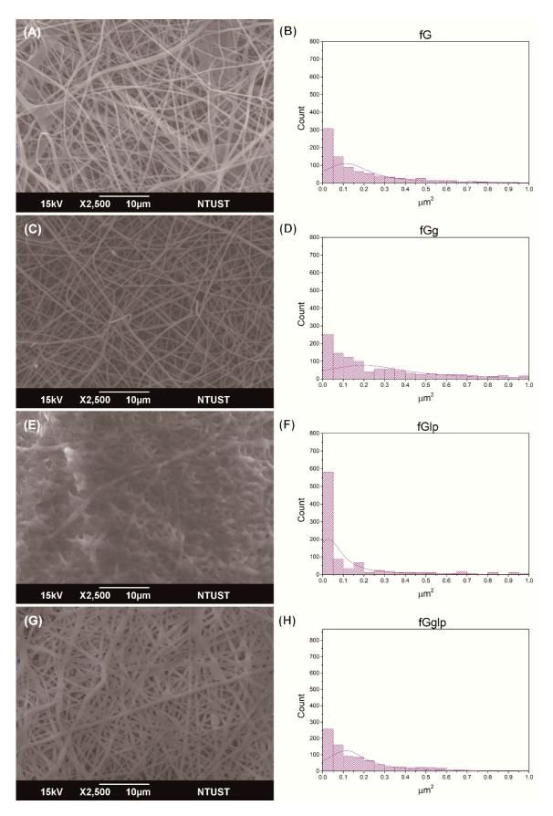
**Figure 1.** The SEM images of indicative nonwoven mat. (**A**,**B**) fG; (**C**,**D**) fGg; (**E**,**F**) fGlp; (**G**,**H**) fGglp. (fG: fish gelatin, g: gallic acid, lp: liquid paraffin).
