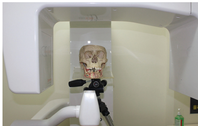
Fig. 1. A dry skull fixed to the tripod for cone-beam computed tomography.
