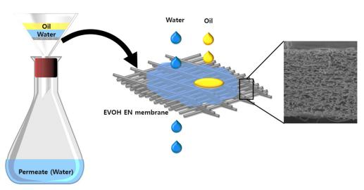
Figure 1. Schematic diagram of the oil/water separation process.
