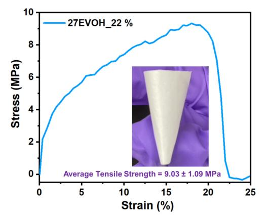
**Figure 7.** Stress–strain curve of the 27EVOH\_22% membrane. The inset is a photograph of the bent electrospun nanofibers.
