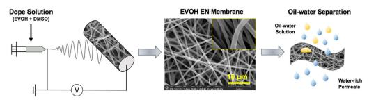
**Figure 2.** Fabrication of the hydrophilic EVOH nanofibrous membrane and its application for oil-water separation.
