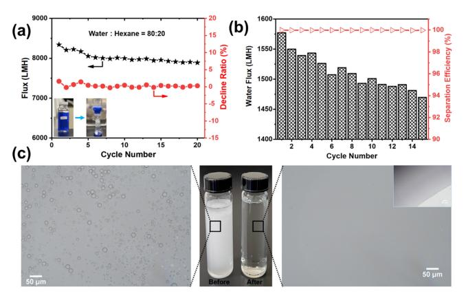
**Figure 9.** (a) Flux recovery and ratio of decline of the EVOH membrane with increasing cycle number. Oil–water emulsion separation results of the 27EVOH\_22% membrane: (b) Flux and separation efficiency of emulsion through the membrane and (c) Optical microscopy images of the emulsion before and after separation. The inset is an image of a permeate water drop near the boundary line.
