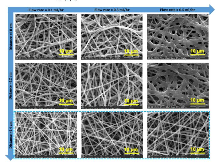
**Figure 5.** FE-SEM images of 27EVOH\_22% at different flow rates and distances used to optimize and study the effect of the electrospinning condition on nanofiber morphology.
