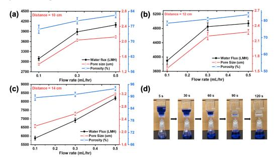
**Figure 6.** 27EVOH\_22% ENM properties at different flow rates and distances between the collector and needle: (**a**) 10 cm, (**b**) 12 cm, and (**c**) 14 cm. (**d**) Visuals of the separation process completed in 120 s.
