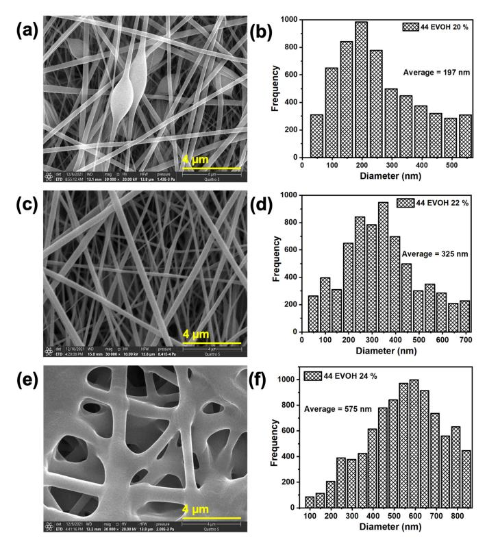
**Figure 3.** SEM images and fiber diameter of 44EVOH at different polymer concentrations: (**a**,**b**) 20 wt%, (**c**,**d**) 22 wt%, and (**e**,**f**) 24 wt%.
