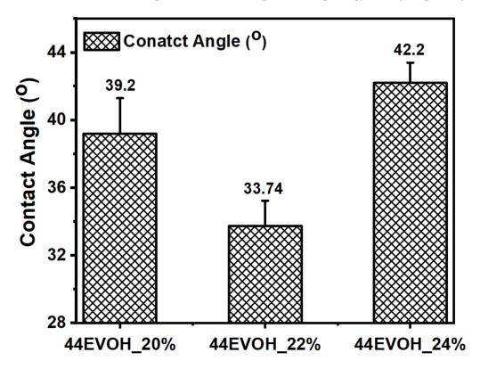
**Figure 4.** Water contact angle of the 44EVOH nanofibers corresponding to the respective polymer concentration.
