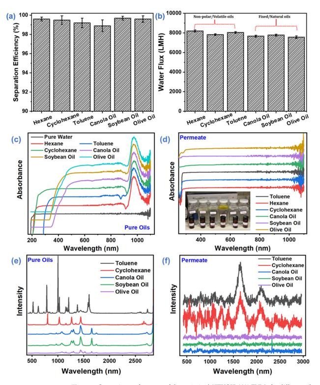
**Figure 8.** Separation performance of the optimized 27EVOH\_22% ENMs for different oil–water mixtures: (a) Separation efficiency, (b) Water flux and UV–visible spectra of pure oils and permeate, (c) Pure oils, (d) Permeates. Raman spectroscopy spectra for pure oils and permeates, (e) Pure oils, and (f) Permeates to confirm separation efficiency >99.9%.
