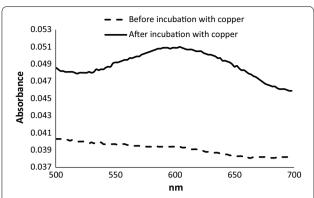
**Fig. 2** Visible spectra of *Sc*Lac before (*dashed line*) and after (*solid line*) incubation with 0.5 mM CuSO<sub>4</sub>. We used 1  $\mu$ M of recombinant enzyme to record the visible spectra between 500 and 700 nm
