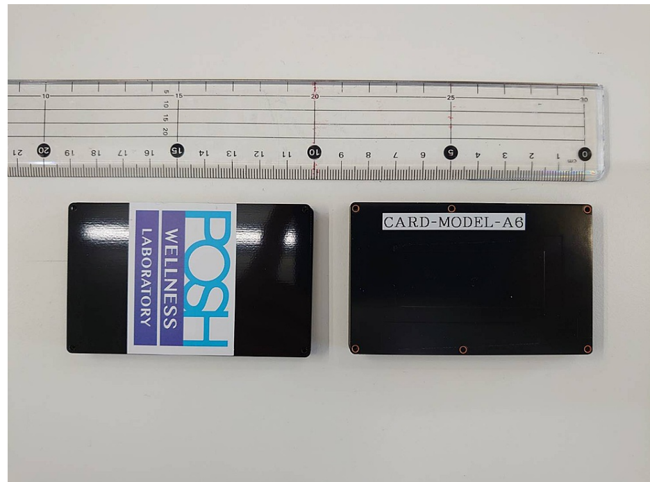
FIGURE 1: Photograph of the developed card-type monitoring device.
