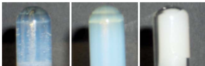
Fig. 8 Polymerization with thermal initiation at 90 °C of (left) 25% F127, 20% PEG5MA, 5% PEG400DA; (middle) 20% F127, 20% PEG5MA, 5% PEG400DA; (right) 20% F127, 40% PEG5MA, 5% PEG400DA (Texter et al. (2006) unpublished)
