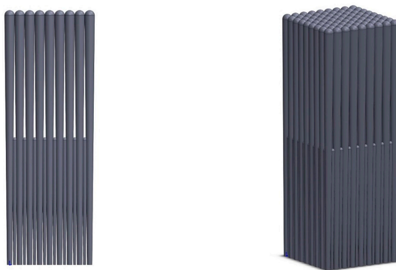
Figure 2. The three-dimensional columnar structure EB-PVD coating model.
