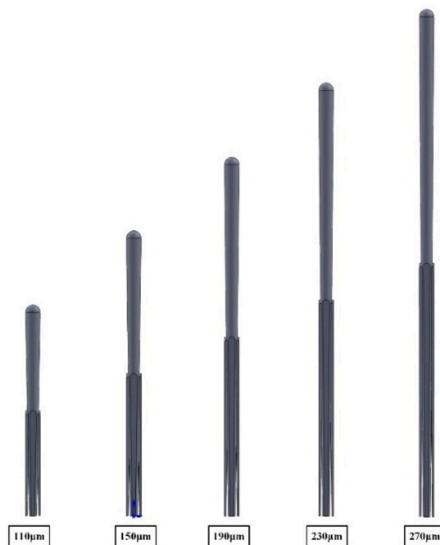
Figure 8. Coating models with different thickness of coatings.
