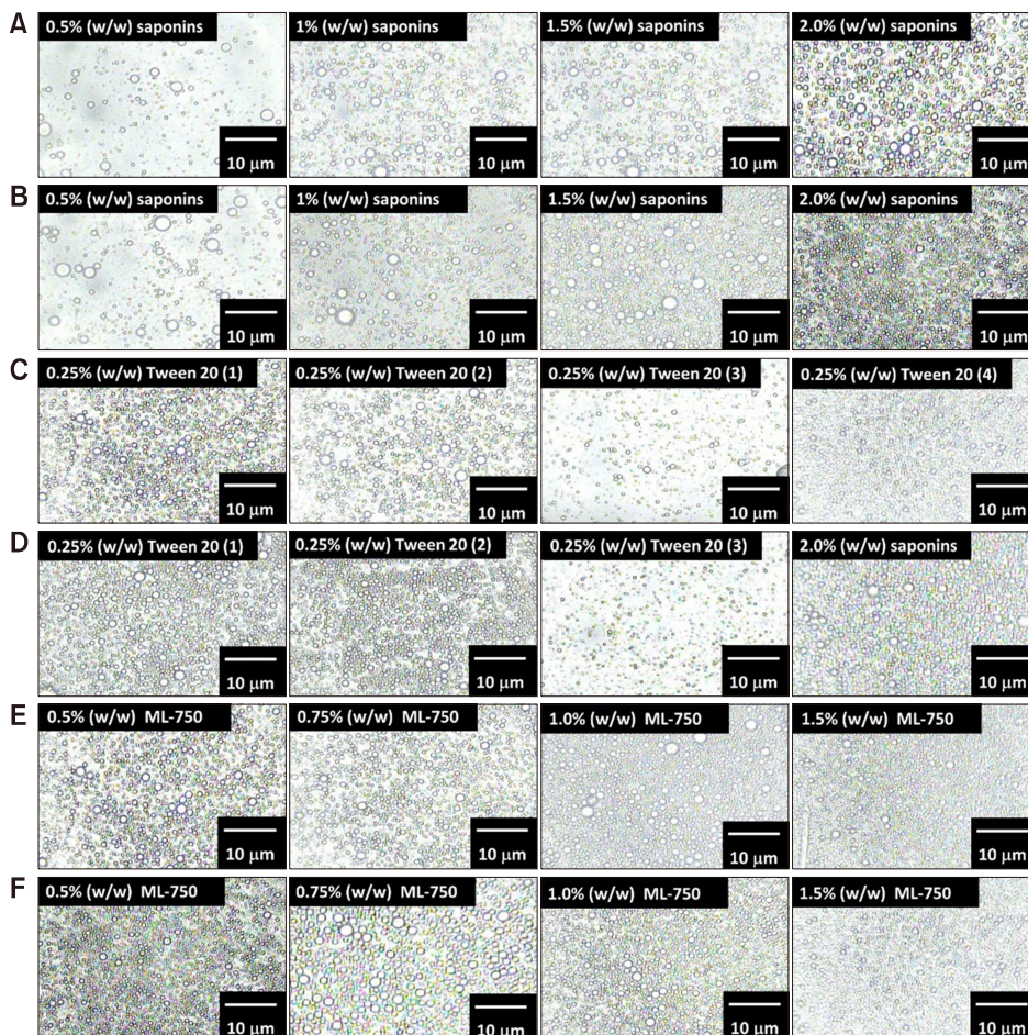
Fig. 2. Optical microstructure representation of different oil in water emulsions. Microstructure of emulsions stabilized with saponin on (A) day 3 and (B) day 7. Microstructure of emulsions stabilized with Tween 20 on (C) day 3 and (D) day 7. Microstructure of emulsions stabilized with ML-750 on (E) day 3 (F) day 7.
