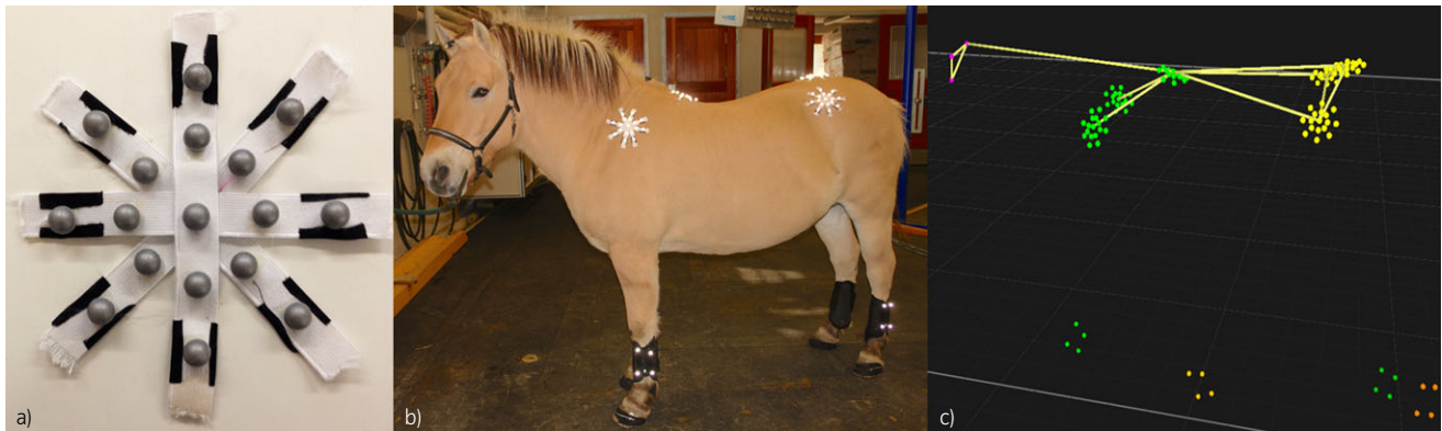
Fig 1: Marker experimental setup. a): Reflective marker cluster construction. b) Marker placement in one of the study subjects. c) Example of left lateral view of all 121 markers as depicted by the 3D tracking software.
