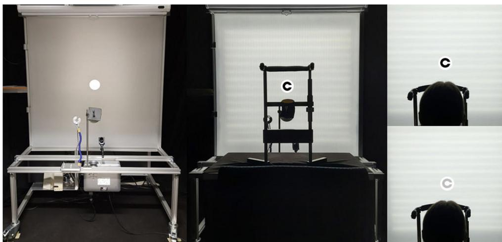
**Figure 1.** Experimental setup (VA-CAL setup, *center*) backlit by computer-controlled LEDs (*left*) generating different ambient luminances. Landolt C-rings can be presented at different contrasts (*right*). The pictures were modified for better visibility of the projected Landolt C-ring.
