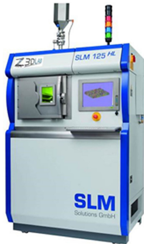
Fig. 6. Photograph of the additive manufacturing machine used to fabricate the studied parts. Selective Laser Melting (SLM) process, model 125 HL , commercialized by SLM Solutions GmbH.
