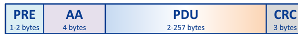
Figure 9. BLE packet structure. The packet has one or two bytes of PRE, depending on the radio data rate, four bytes of AA, from two to 257 bytes of PDU and three bytes of CRC.
