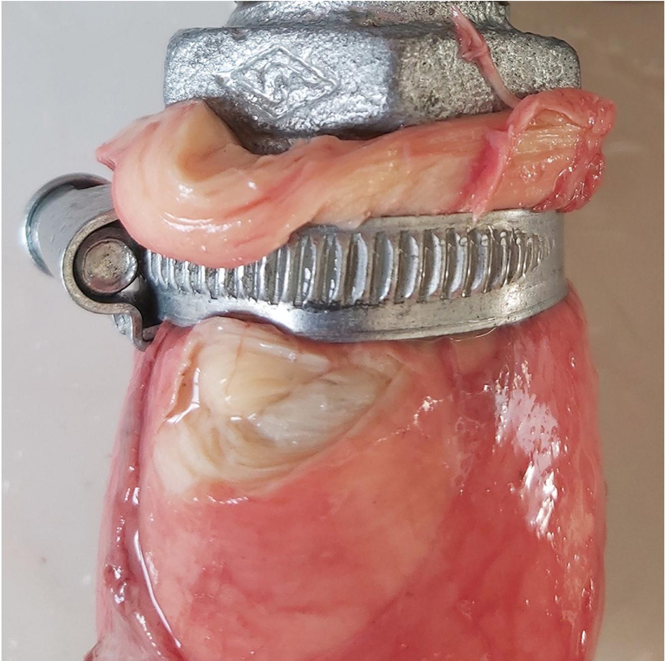
**Fig 7. Typical cross-sectional rupture of the proximal aorta, close to the mounting side, which occurred predominantly in older horses (> 15 years) at high pressures (250–300 mmHg).**
