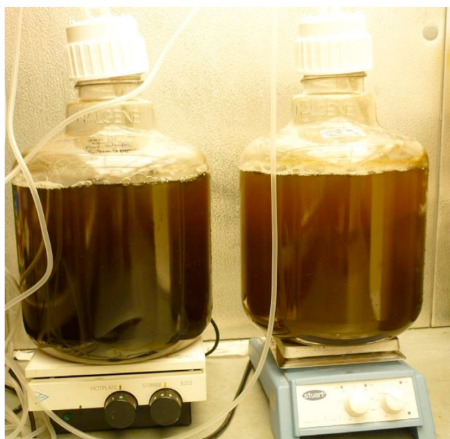
Figure 1. Set-up showing cultivation of Amphora sp. inside the environmental growth chamber at 20 °C, under 45–80 μmol photons m -2 sec -1 illumination with 16/8h light/dark cycle, and micro-filtered aeration (0.8 L/min) through aquarium pump.
