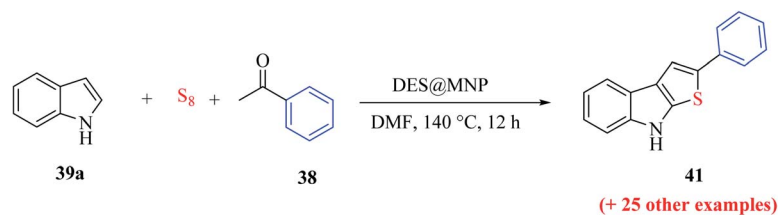
Scheme 52 Synthesis of 2-phenylthieno[2,3- b ]indole 41 from DES@MNP.
