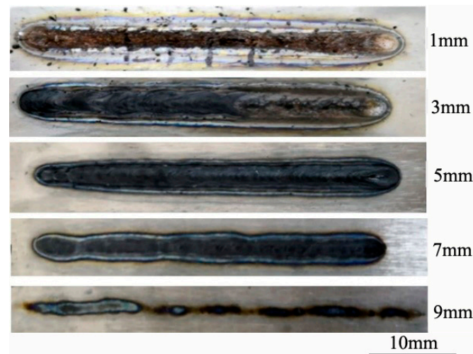
Figure 2. Macroscopic morphology of wet laser welding seam under different water depths.
