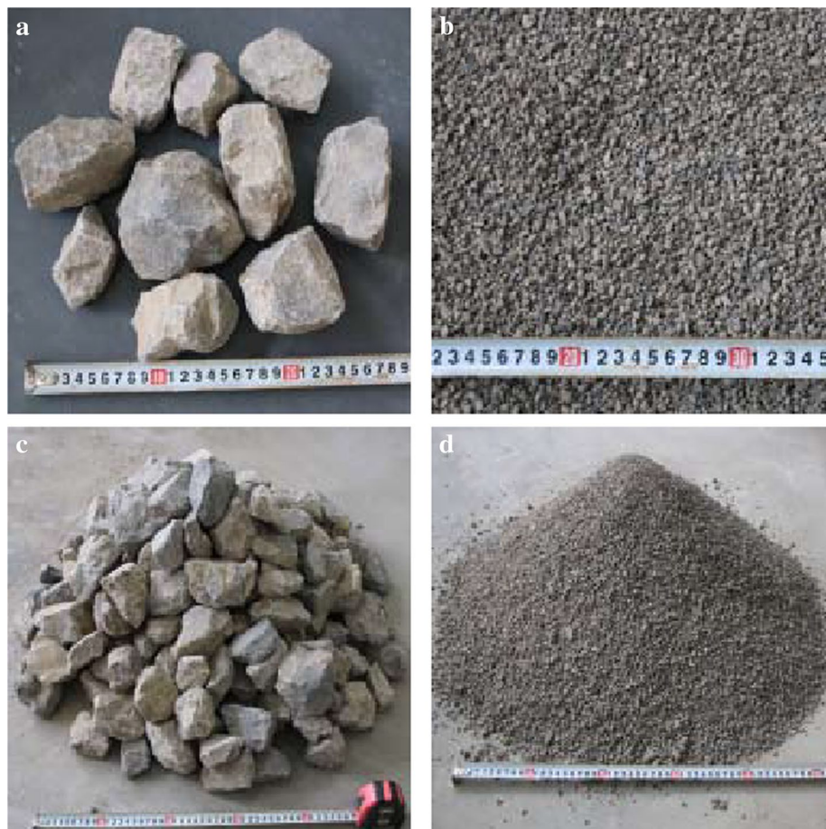
Fig. 2 Fragment materials used for the laboratory tests: a 40–80 mm; b 2–5 mm; c repose angle of the debris avalanche materials and d repose angle of the substrate materials
