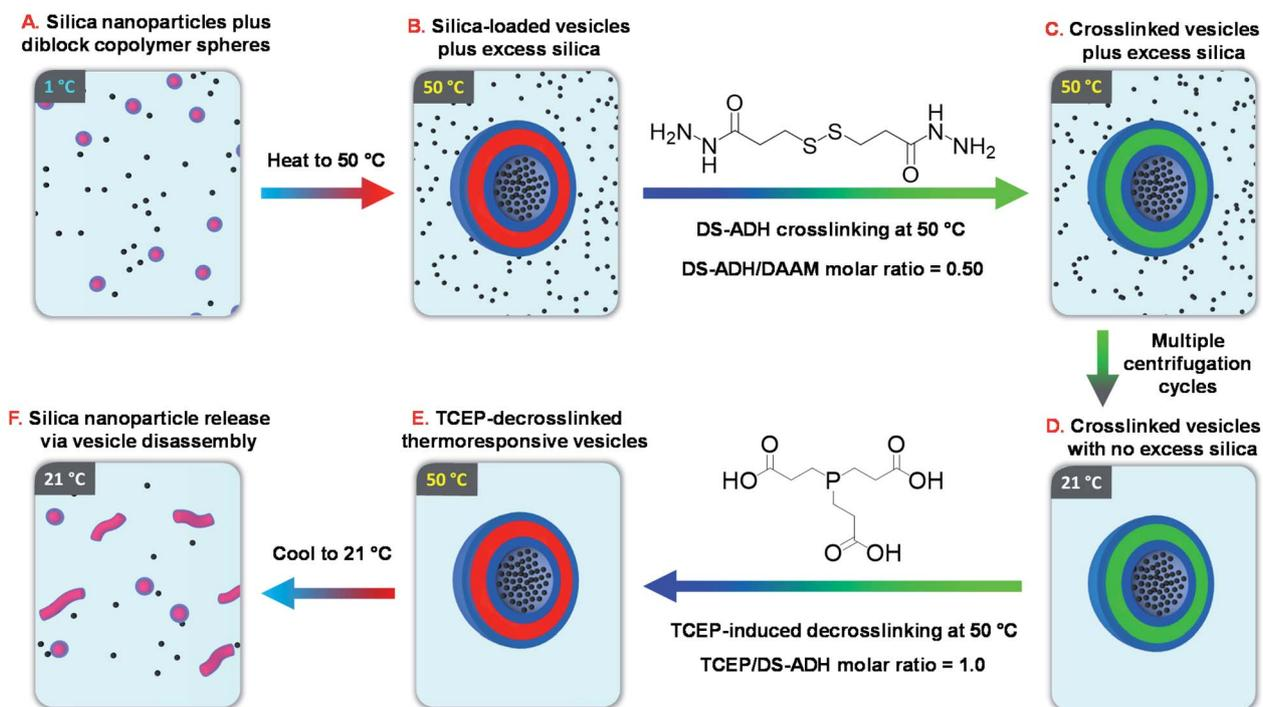
Fig. 1 Schematic overview of the six stages involved in the encapsulation and release of silica nanoparticles using a thermoresponsive ‘shape-shifting’ PDMAC<sub>56</sub>-P(HBA-*stat*-DAAM)<sub>254</sub> diblock copolymer.
