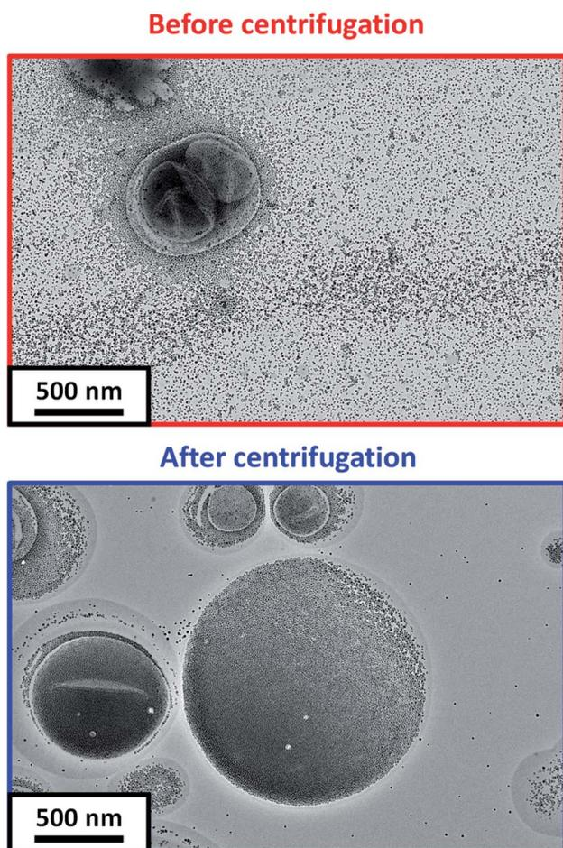
**Fig. 4** Representative TEM images recorded for DS-ADH crosslinked PDMAC<sub>49</sub>-P(HBA-*stat*-DAAM)<sub>302</sub> vesicles prepared at a copolymer concentration of 5.0% w/w in the presence of a 20% w/w aqueous dispersion of silica nanoparticles (a) before and (b) after ten centrifugation–redispersion cycles to remove excess silica nanoparticles.
