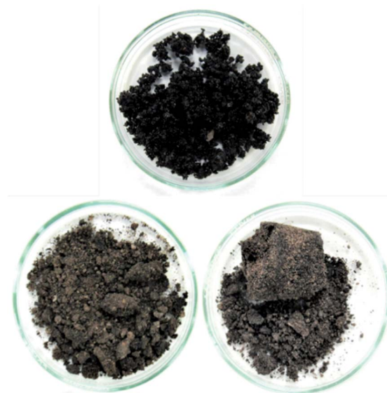
Fig. 7 Dynamic test 2 sand pack: top – original sand sample; bottom left – inlet sand sample after test, and; bottom right – outlet sand sample after test.
