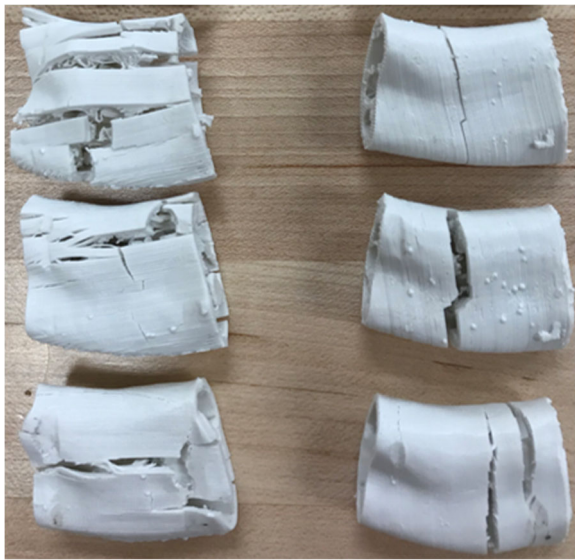
Fig. 14 Comparison of failed grafts with round-pore, square-pore and topological optimized-pore scaffold structures, from top to bottom printed at 0-degree (left) and 90-degree (right)
