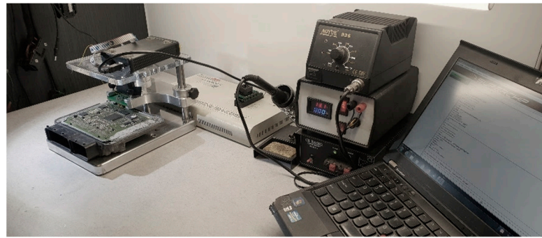
Figure 3. Stand for modification of vehicle computer software.
