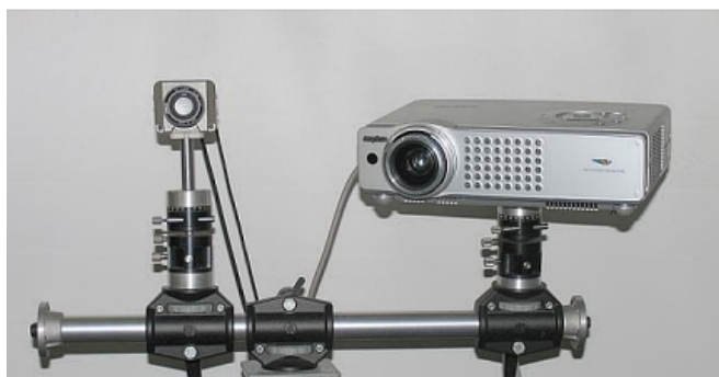
Figure 13. The low-cost whole-field structured light sensor designed for modeling applications.
