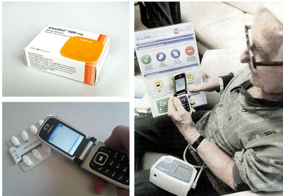
FIGURE 1 Data collection via near-field communication (NFC). Left top: medication packaging with attached NFC tag; left bottom: collecting data from a smart blister; right: collecting data via NFC by touching a blood pressure meter and the fields of a chart, which are equipped with NFC tags. (© AIT Austrian Institute of Technology GmbH)
