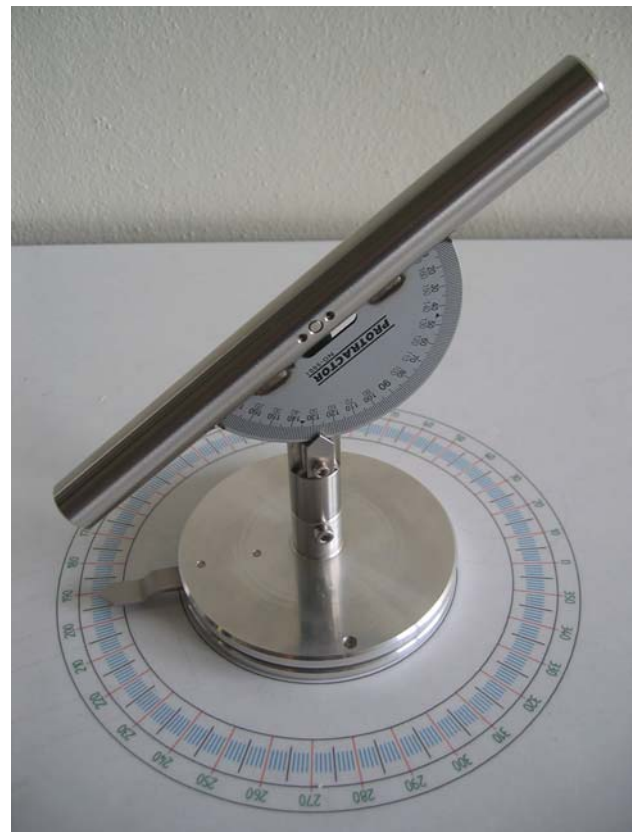
Fig. 4 A close-up of the bar used in the experiment with the half protractor on the bottom of the bar indicating the tilt ( \theta ) and with the protractor at the base of the pole indicating the slant ( \varphi )
