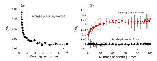
**Figure 3.** (a) Relative changes in the resistance of the PVOH/ $Bi_2Se_3$ -MWCNT composite with 30 wt.%  $Bi_2Se_3$ -MWCNT filler vs. its bending radius (R is the resistance of the bent composite,  $R_0$  is the resistance of the composite before the first bending cycle); (b) relative changes of the resistance of PVOH/ $Bi_2Se_3$ -MWCNT composite with 30 wt.%  $Bi_2Se_3$ -MWCNT filler under repetitive bending down to 10 mm (black dots) and 3 mm (red dots) vs. bending radius.
