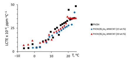
**Figure 4.** Linear coefficient of thermal expansion (LCTE) vs. temperature of neat PVOH and PVOH/Bi<sub>2</sub>Se<sub>3</sub>-MWCNT composites.
