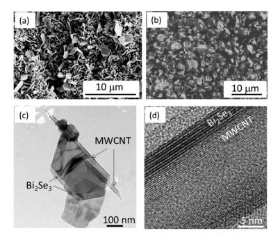
Figure 1. (a) Scanning electron microscopy (SEM) image of as-grown  $Bi_2Se_3$ -MWCNT (multiwalled carbon nanotube) hybrid structures with ratio 90 wt.%  $Bi_2Se_3$ : 10 wt.% MWCNT; (b) SEM image of the surface of polyvinyl alcohol (PVOH)-based composite with 30%  $Bi_2Se_3$ -MWCNT filler; (c) transmission electron microscope (TEM) image of a  $Bi_2Se_3$ -MWCNT hybrid structure; (d) High-resolution TEM image of  $Bi_2Se_3$ -MWCNT interface.
