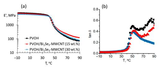
**Figure 6.** (a) Storage modulus and (b) tan  $\delta$  vs. temperature relationships of various PVOH-based composites.
