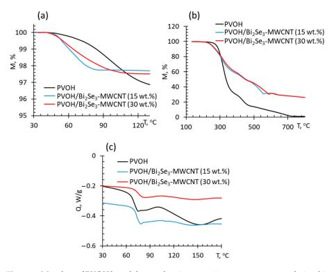
**Figure 5.** Mass loss of PVOH based thermoelectric composites vs. temperature relationships, recorded at oxidative environment within temperature diapason between (a) 30-130 °C and (b) 130-700 °C as well as differential scanning calorimetry thermograms obtained after the removal of thermal history of the samples (second run of measurements) (c) of various PVOH-based composites.
