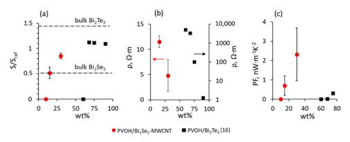
**Figure 2.** Comparison of the properties of the PVOH/ $Bi_2Se_3$ -MWCNT composites (red dots, this work) with the properties of PVOH/ $Bi_2Te_3$  [16] (black squares) composites vs. filler wt.%: (a) Seebeck coefficient of the composite (S) relative to the Seebeck coefficient of the nanostructured materials ( $S_{ref}$ ) [16,22,26–29]; (b) resistivity; (c) power factor.
