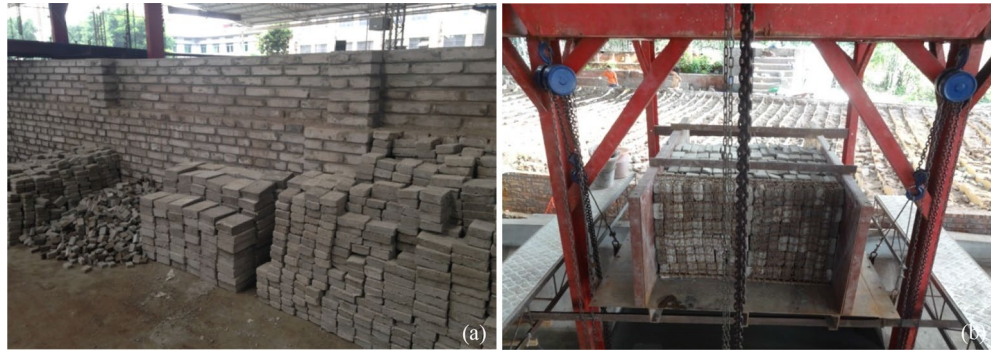
Figure 2. (a) Rigid concrete blocks; and (b) landslide model assembled with rigid blocks.
