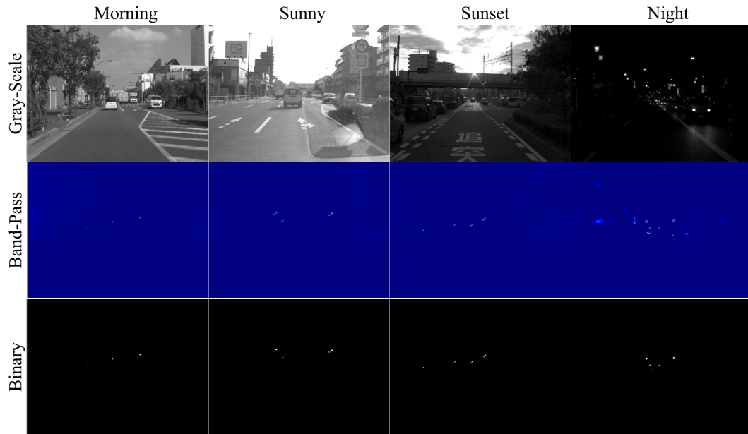
Figure 9. Intermediate results in all scenes. Each column corresponds to a scene. The upper row shows the gray-scaled images, the middle row displays the band-pass-filtered images, and the lower row illustrates the binarized images.
