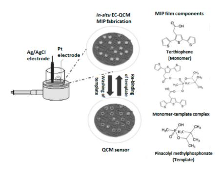
Figure 9. MIP-based QCM sensor toward pinacolyl methylphosphonate (reproduced with permission from [59]).
