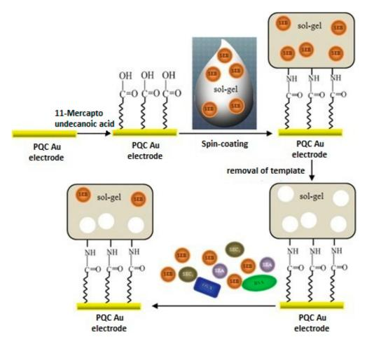
**Figure 3.** Schemes of the preparation of sol-gel imprinted thin film on the surface of the piezoelectric quartz crystal (PQC) Au-electrode for the detection of staphylococcal enterotoxin B (SEB) (reproduced with permission from [19]).
