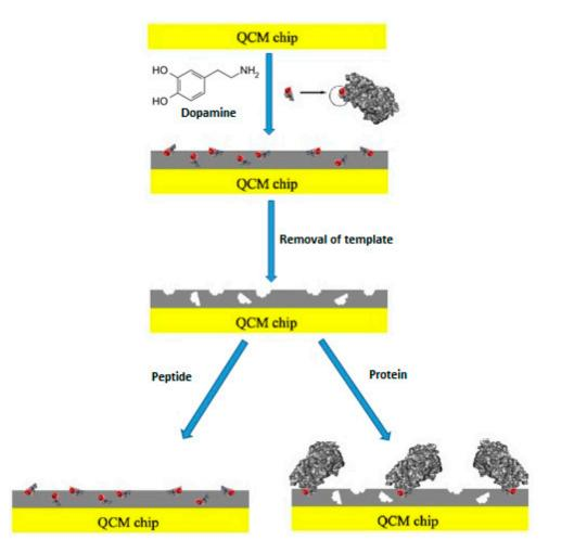
Figure 4. Schematic representation of epitope-imprinting (reproduced with permission from [20]).
