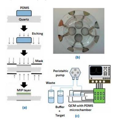
**Figure 5.** (a) Schematic demonstration of MIP-based QCM sensor; (b) Prepared MIP based-QCM sensor with multi-channel; (c) Schematic depiction of the prepared sensor system combined with impedance analyzer (reproduced with permission from [28]).
