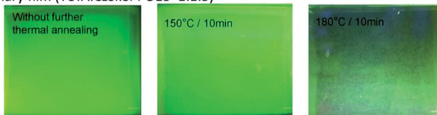
Fig. 8 Photographs of (a) binary films and (b) ternary films under UV irradiation.
