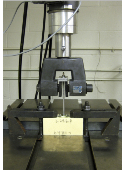
Fig. 2. Pullout testing setup.
