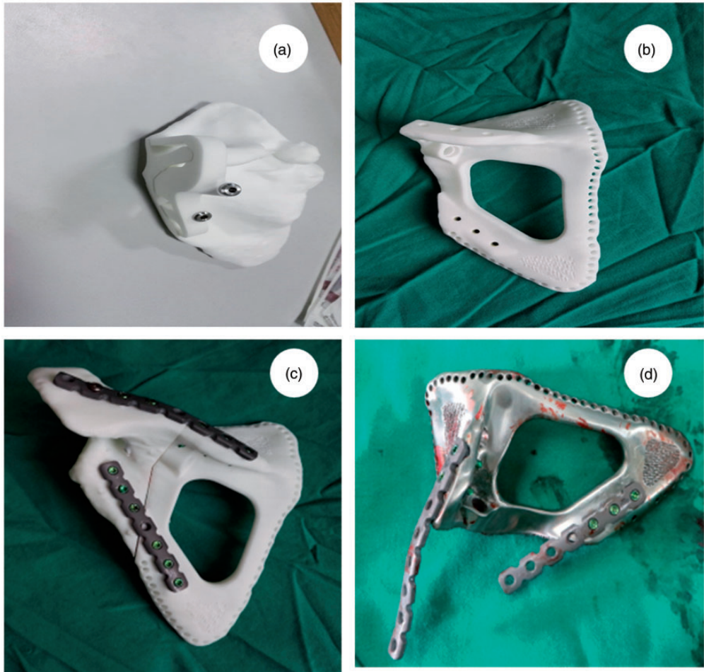
Figure 3. Solid three-dimensional model of the left scapula and preoperative simulation. (a) A navigation template stuck to the removed portion of the scapula (S1). (b,d) The nylon and titanium alloy prostheses (N-S1) were printed using mirror imaging technique. Many holes were designed at the edge of the prosthesis for soft tissue reconstruction. (c) The retained portion of the scapula (S2) and the prosthesis (N-S1) matched well via the reconstruction plate shaped in advance.
