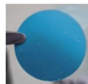
Scheme 2 Synthesis of [\text{Cu}(1,3\text{-YBDC})] \cdot x\text{H}_2\text{O} and image of a pellet made by pressing at 100 bar for 2 min its polycrystals.
