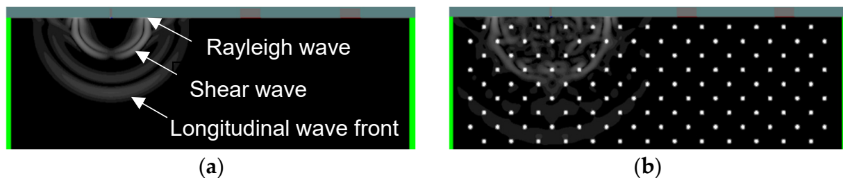
Figure 4. Displacement field close to the surface of (a) mortar without voids and (b) mortar with 3% voids a few \mu\text{s} after excitation.
