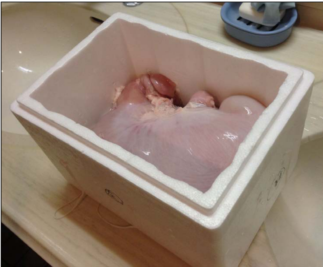
Fig 4. The stomach model was filled with 500 mL of water and fixed in a styrol-foamed box to allow it to rotate manually.
