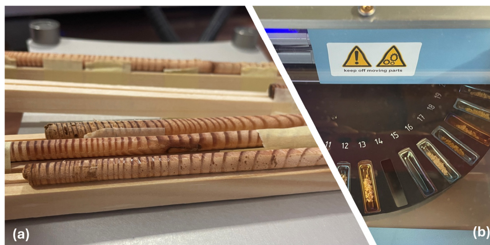
Figure 2. Methodology for dendrochronological Hg analysis. (a) Tree cores prepared for annual ring dating and measurement using a precision measuring stage. (b) Thermal Decomposition Amalgamation Atomic Absorption Spectroscopy (TDA-AAS) system (Milestone DMA-80® Tri-Cells) for direct quantification of Hg in wood samples.
